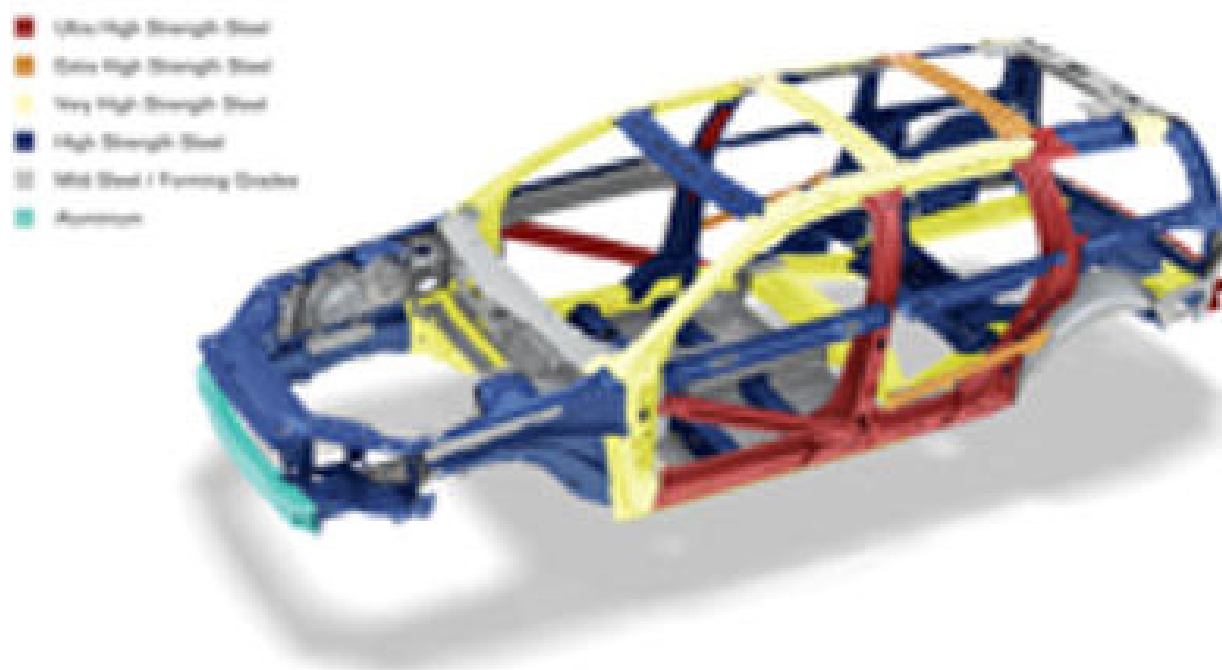
Drawing showing different kinds of metals in the Volvo’s frame.
